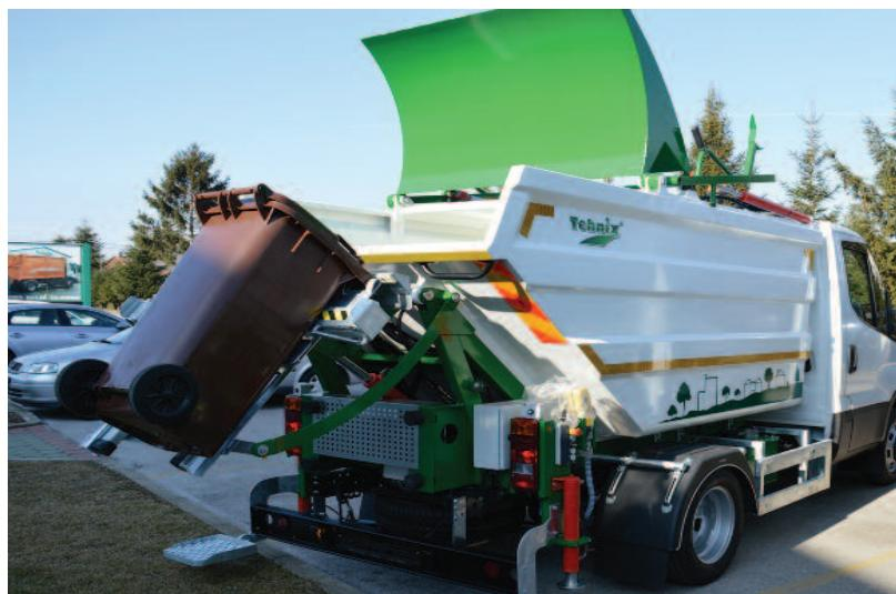
Pražnjenje posuda zapremnine 80 do 1100 litara / Discharge of bucket container 80 to 1100 liter capacity
