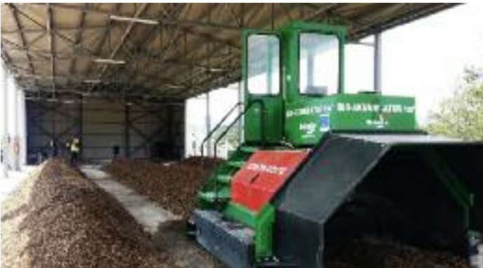
COMPOST SHREDDER - AUTOMATIC WITH CRANE - TYPE TEHNIX DIESEL 130 KW
