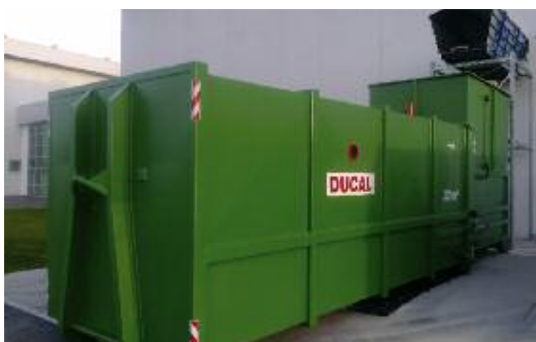
Special desing of two-part press-container with lifter
