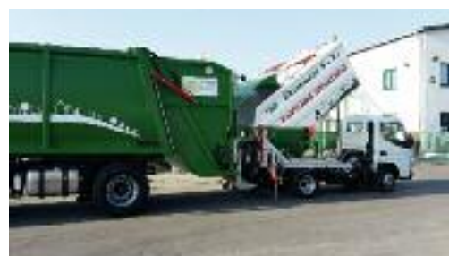
Collected municipal waste is reloaded from a smaller vehicle into a larger one
