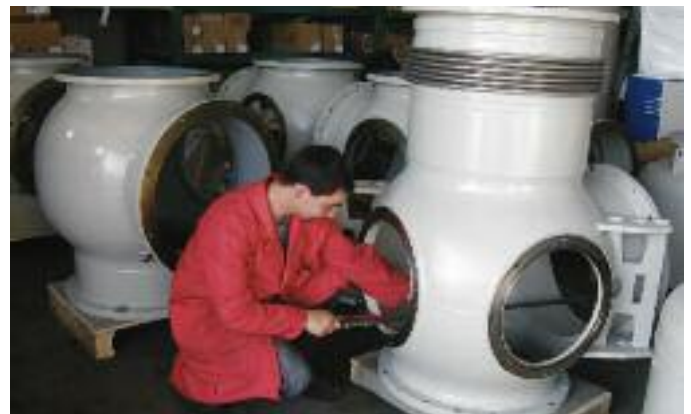
Final control of finished casings after painting
