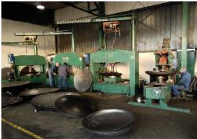
Production of floors from 15 mm thick tin sheets and diameter from 500 to 3000 mm according to norm DIM 28011 (shallow) and DIN 28013 (deep)
