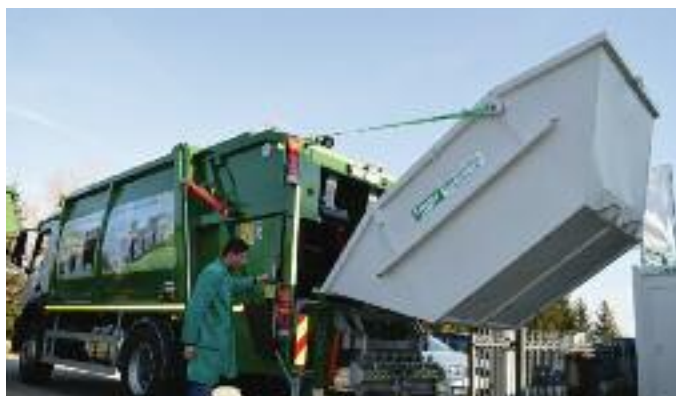
Tehnix skip loader for containers 5 and 7 m 3
