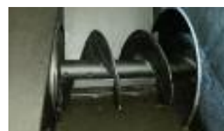
Driving worm, high pressing efficiency (1:10)
