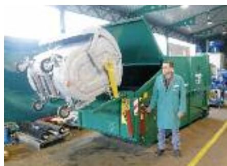
Hydraulic press-container with lifting unit
