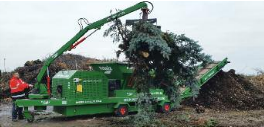
COMPOST SHREDDER - AUTOMATIC WITH CRANE - TYPE TEHNIX DIESEL 130 KW
