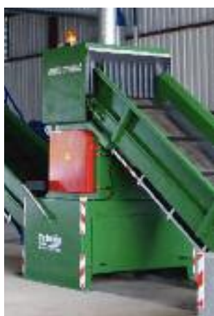
Bags opener type TEHNIX - capacity from 5-20 t/h, possibility of bags opening 5-50 kg
