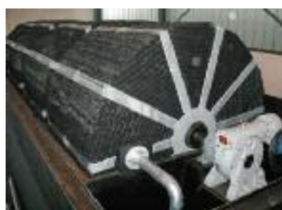
Rotor of biological section of device
