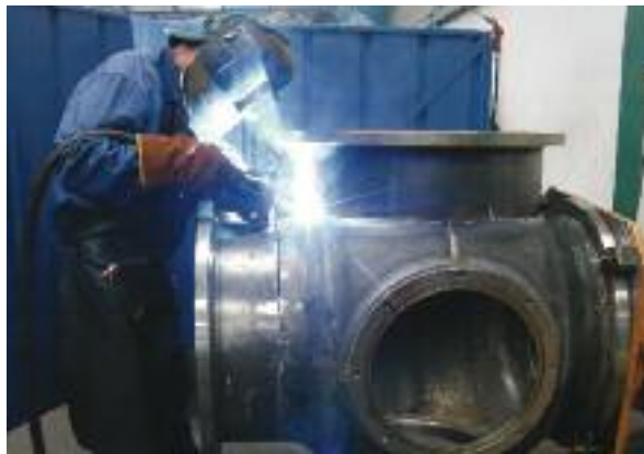
Preparation and welding of special casings
