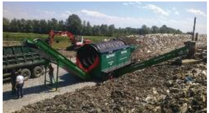
SANATOR OF OLD DUMPS TEHNIX Extraction of compost
