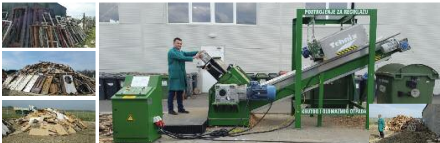
Shredder for shredding of wooden, plastic and rubber waste with electromagnet for metal extraction
