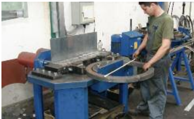
Flanges production by bending on special machine
