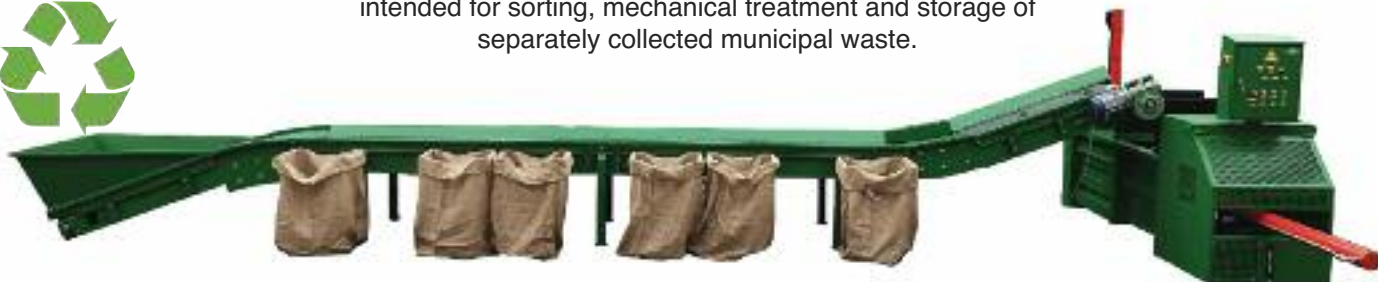
MANUAL SORTING FACILITY TYPE TEHNIX CAPACITY UP TO 1 t/h BALING OF RAW MATERIALS IN BALES WIRE-STITCHED WITH VPB-20 WITH 4 OR 6 WORKING PLACES
