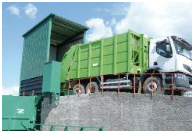
Automatic reloading station type Tehnix - from garbage truck to 32 m³ press-containers
