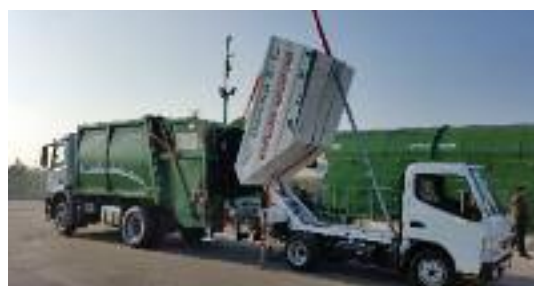
Collected municipal waste is reloaded from a smaller vehicle into a larger one
