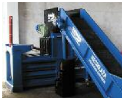
Press with a transporter and perforator of PET packaging
