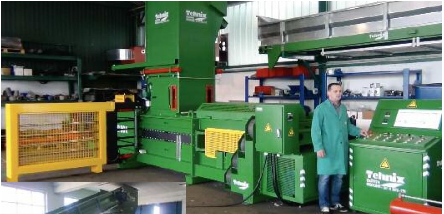
Automatic baling press with additional equipment and control panel
