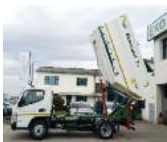
Collected municipal waste is reloaded from a smaller vehicle into a larger one
