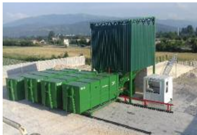
Automatic reloading station type Tehnix - from garbage truck to 32 m³ press-containers
