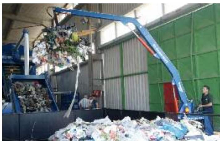
TEKRAN TEHNIX - for dosing of mixed communal waste
