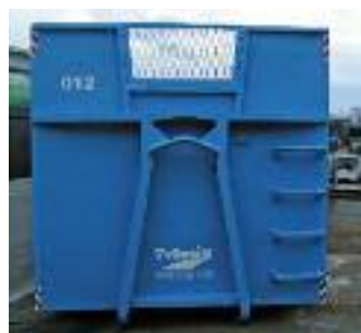
Rolo container with crane opening
